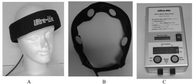
A B C Figure 1. Low-intensity, low-frequency pulsed ultrasonic device. A. Depiction of how the transducer headband was worn by participants. B. The position of the ultrasound transducers in the headband (Type B). C. Transduction control device
